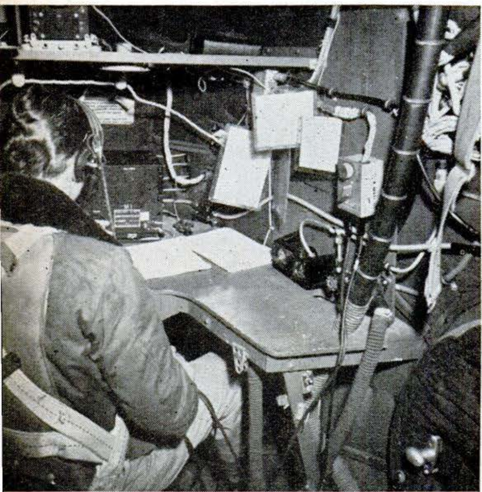
System requires no special equipment in plane. Using standard AN/ARC-8 liaison transmitter-receiver installed in all Air Force aircraft, operator has world-wide radio coverage.
